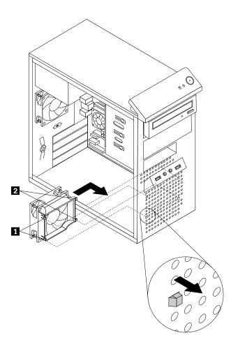
Figure 42. Installing the front fan assembly
